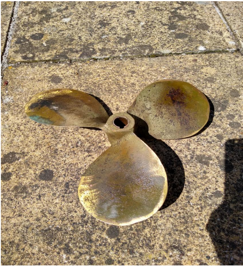
Reconditioned bronze Boat propeller. 16 ins dia, 12 ins pitch, right hand, for a inch and a quarter shaft For sale at £50.
